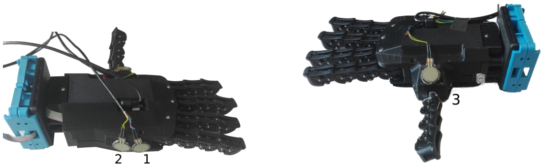
Figure 2.1: Pisa/IIT SoftHand with FSR sensors for handshake
